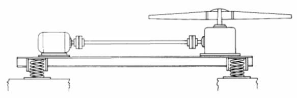
Figure 6 Schematic of Vibration Isolation Mounting for Fan and Drive-Assembly of Propeller-Type Cooling Tower
