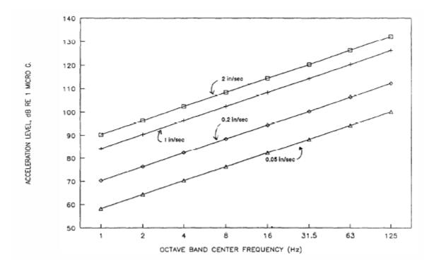
Figure 2 Vibration Criteria for Damage Risk to Buildings.
